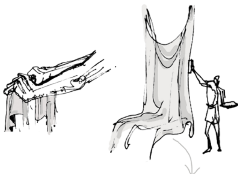
Repeated experimentation of Kora cloth (waste cloth) finished with a layer of ferrocement and then grey oxide, with further waxing and polishing led to the making of the CLOTHCRETE partitions that were only an inch thick but still retained all the undulations and beautiful folds of falling drapes.
